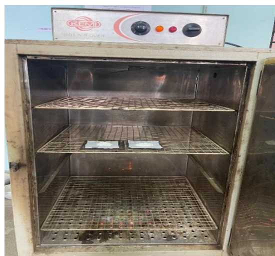
Figure No: 12 Drying of powder in hot air oven
